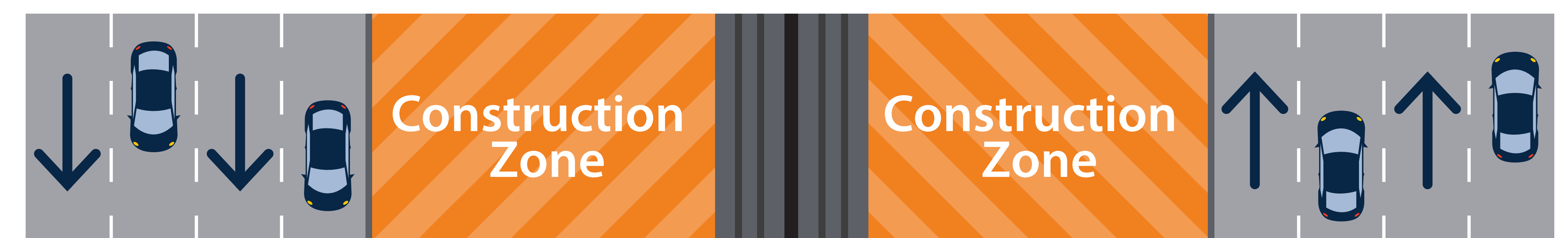
Phase 2: Traffic is shifted to the outside of the corridor
