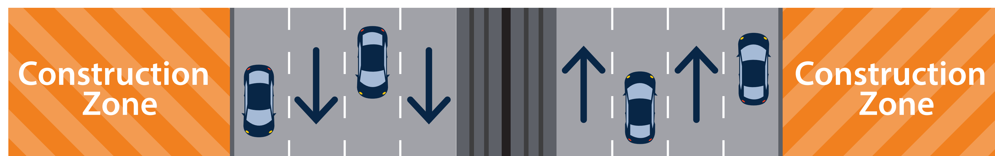
Phase 1: Traffic is shifted to the inside of the corridor
