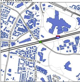
**Project Description:** Add a sidewalk on the west side of the existing bridge with a signalized crosswalk at the new ramp to the Managed Lanes (westbound).
